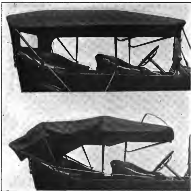
Fig. 4—Ohio Top hoist in use. Fig. 5—Being dismantled
